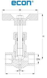
Econ® needle valves, especially suitable for accurate regulation of gases and liquids. Not suitable for steam.
